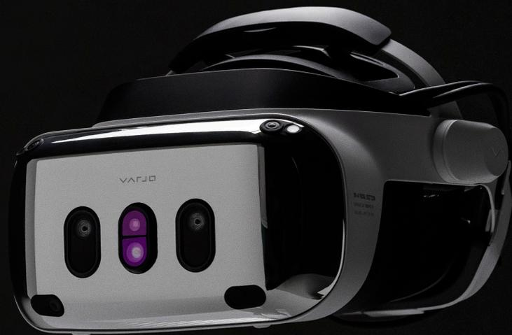
Dual 20-megapixel front mounted cameras and autofocus system improve near and far field vision and create the industry's best mixed reality experience.
